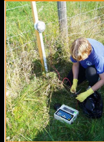
Measuring current in a buried pipeline.
